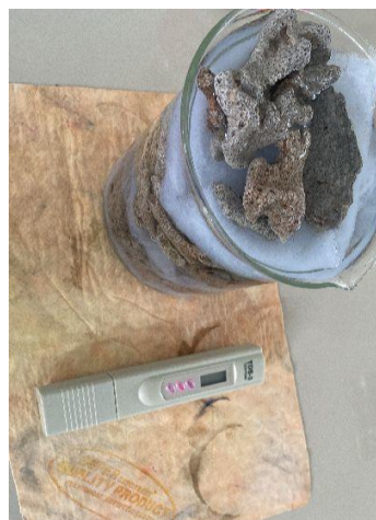
Proses Pengukuran kadar TDS
